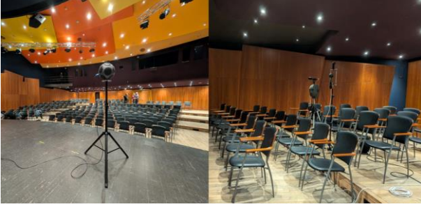
Fig. 3. Position of the sound source (left) and the equipment setup (right) during the acoustic measurements.
